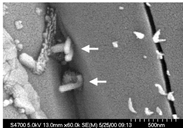
Figure 5. SEM images of the fractured Y-Ba-Cu-O/MWNTs composite disk. (a) Some rods were seen to protrude from the fracture surface. (b) Some rods were bridging between two sides of microcracks on the surface of the Y-Ba-Cu-O/MWNTs composites disk.
